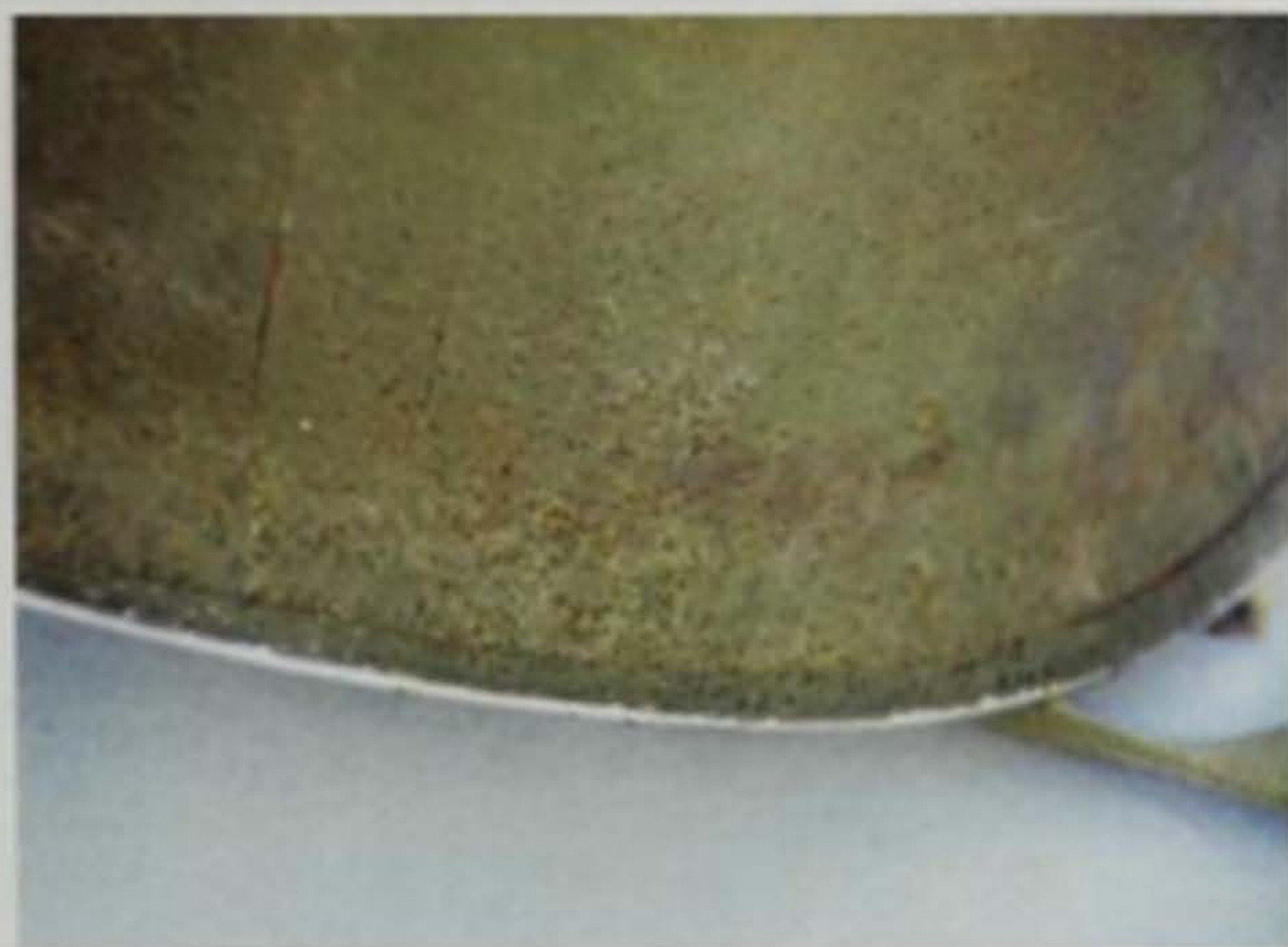
Exterior view of the M-1 helmet body exterior finish, ca. 1941-1945. Note the cork aggregate applied to the olive drab exterior paint.
