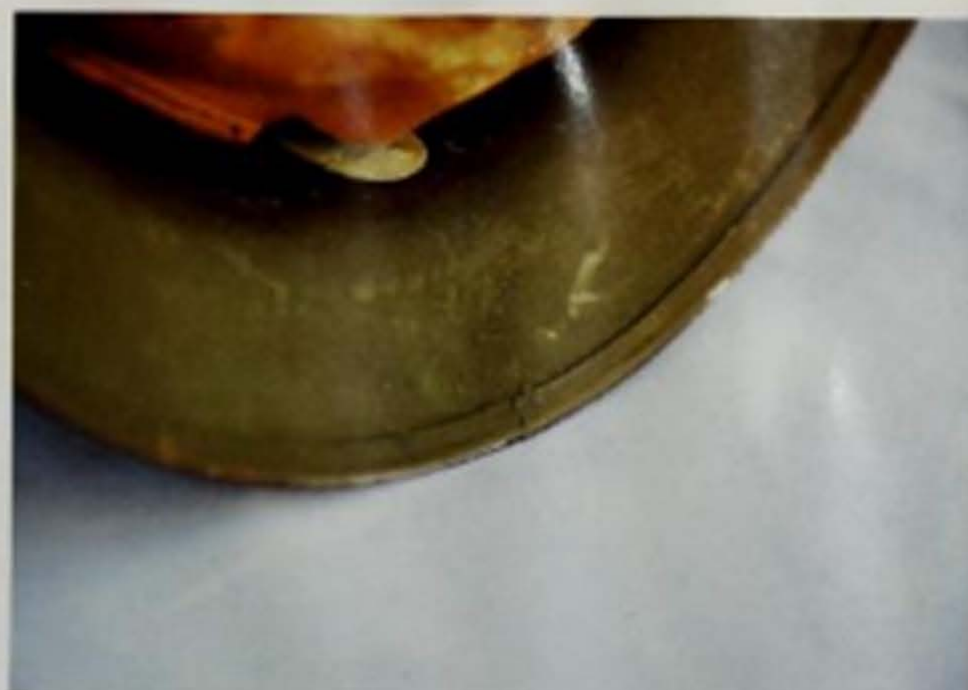
Close-up of the production M-1917A1 stamp marking, ca. 1940. The stamp was placed under the brim of the helmet and represented a heat and shipment number. This view also shows the edging butt.
