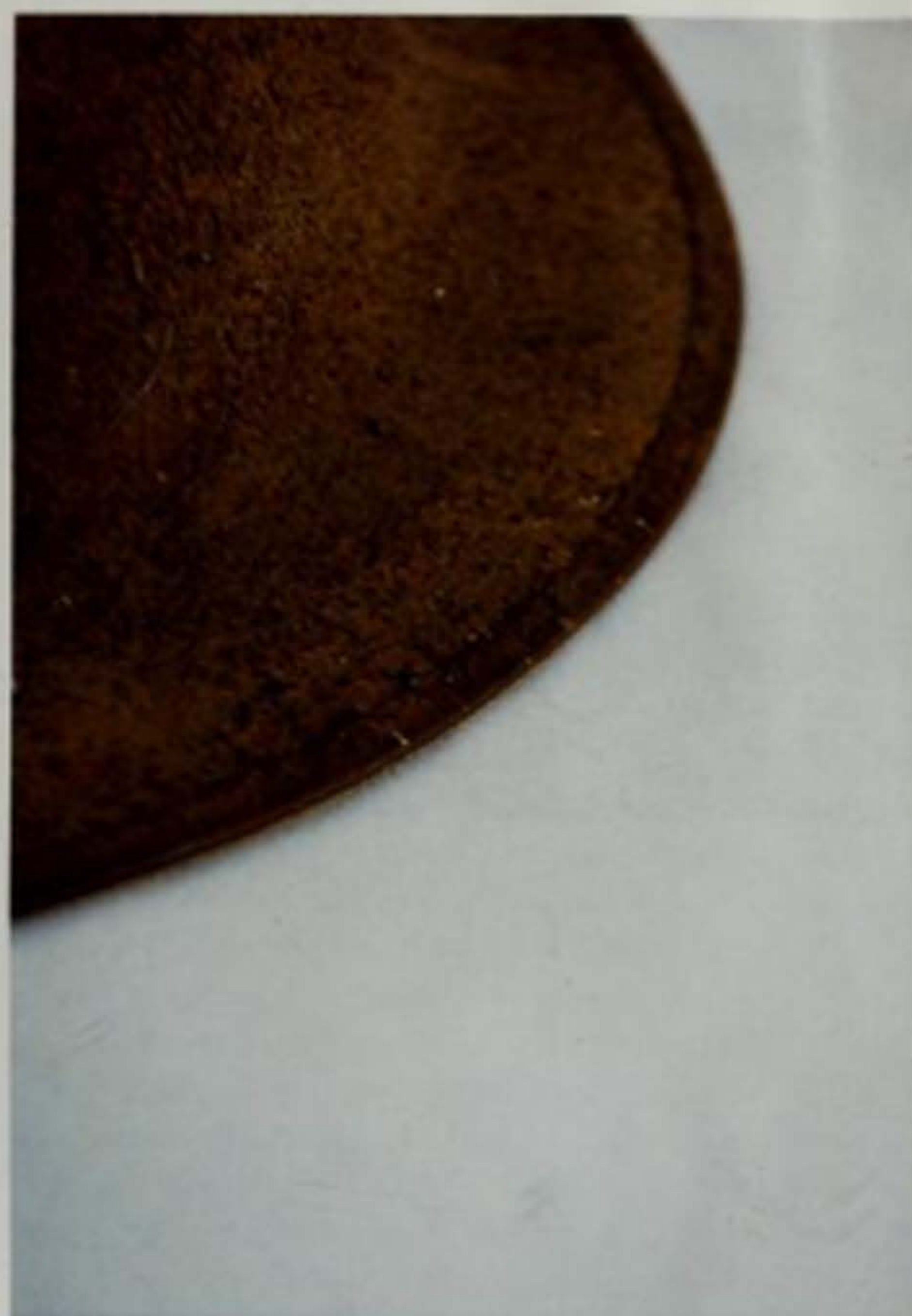
Close-up of the M-1917 exterior finish, ca. 1917-1918. This view shows the sawdust aggregate applied to the olive drab finish.
