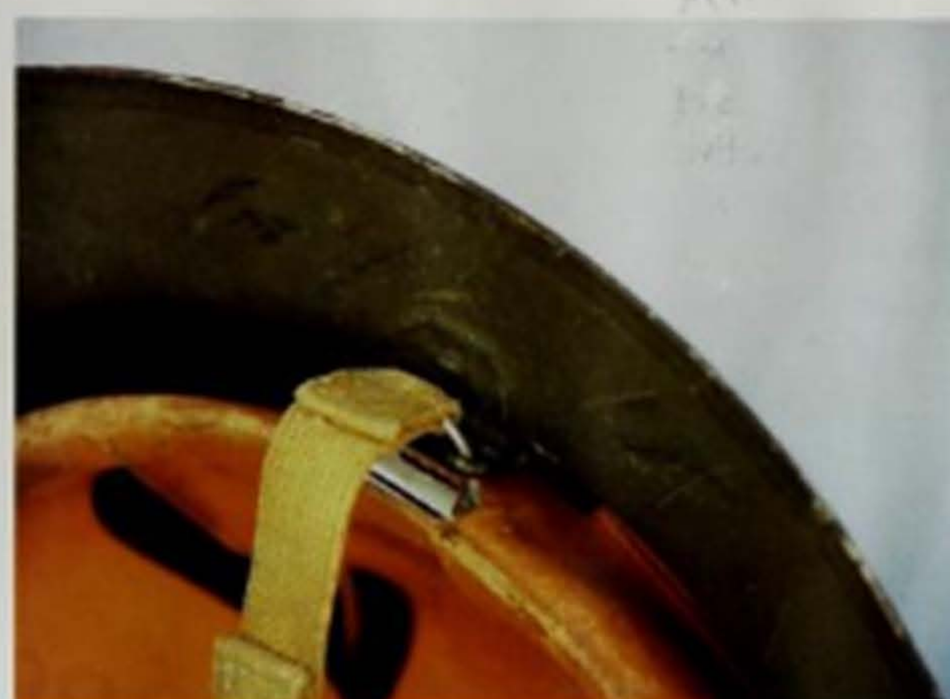
Production M-1917A1 chin strap loop, ca. 1940. Note the machined rivet used to secure the loop to the helmet. Additionally, note the webbed chin strap attached to the suspension as opposed to the loop itself.
