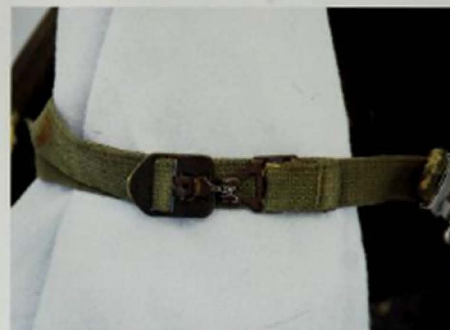
Fastened M-1 helmet body chin strap buckle and release hook, ca. 1961-1963. The buckle was stamped of brass coated with a mildew inhibitor.
