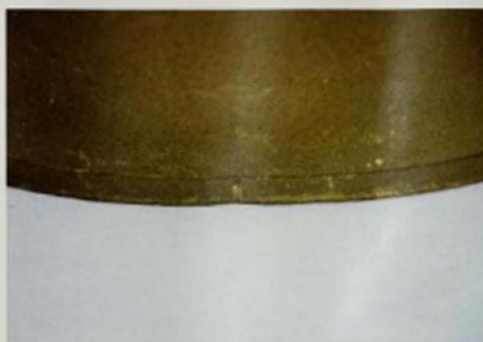
Exterior view of M-1 helmet body rear edging butt, ca. 1951-1960. Note the sand aggregate applied to the exterior paint.
