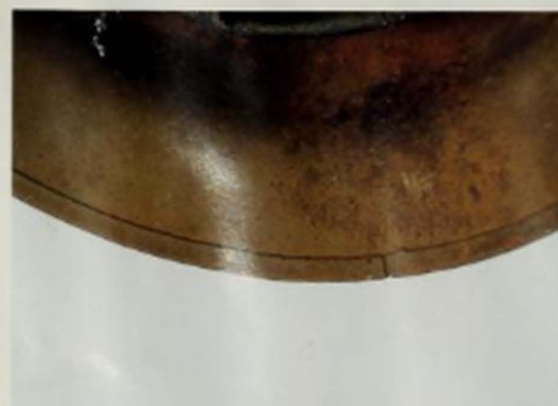
Close-up of the M-1917 stamp marking, ca. 1917-1918. The stamp was placed under the brim of the helmet and represented a heat and shipment number.
