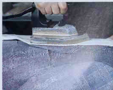
The suit is pressed throughout the process of making up. In Italy, as in England, the last pressing gives it its final shape.
