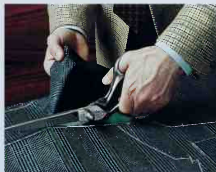
Cutting by hand is an important stage in making top-quality clothing. It makes the most economical use of the fabric and guarantees that the patterning will match.
