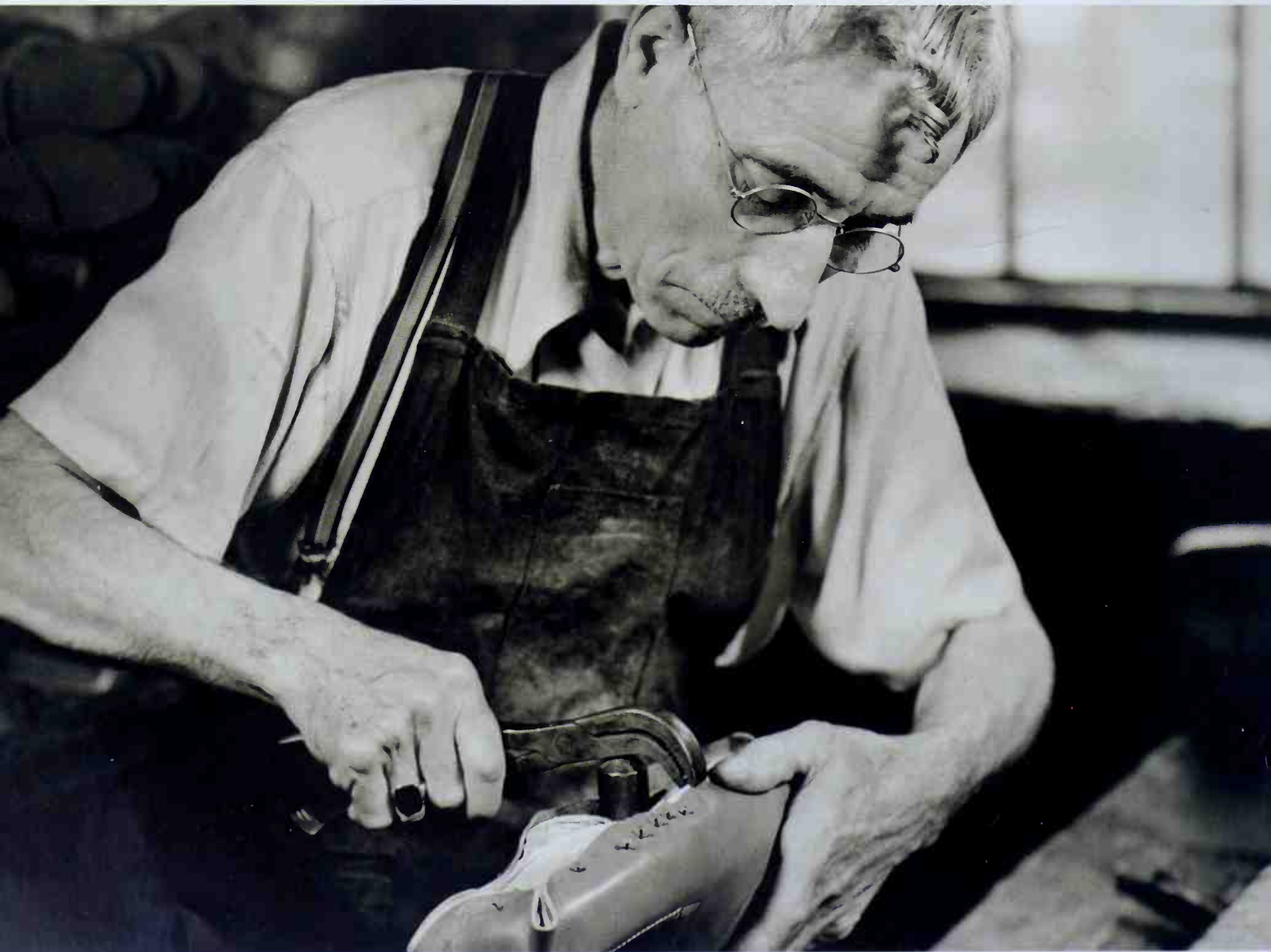
The times when the upper used to be stretched over the last by hand at Alden are long past. Today this process is carried out using a machine, but this has no effect on quality.
