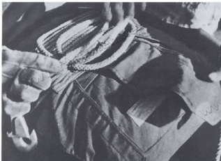
Above: Detail showing the static line on an RZ1 parachute, the original Göring parachute that was superseded by the RZ30.
