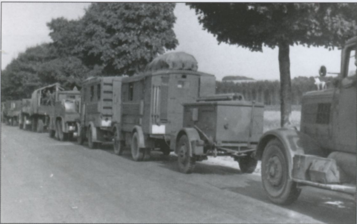
Signals units possessed more specialized vehicles than any other type of unit. Various types of radio trucks (Funkkraftwagen) are seen here with sectional antenna racks on their sides. The trailer contains a heavy power generator (schwerer Maschinensatz).
