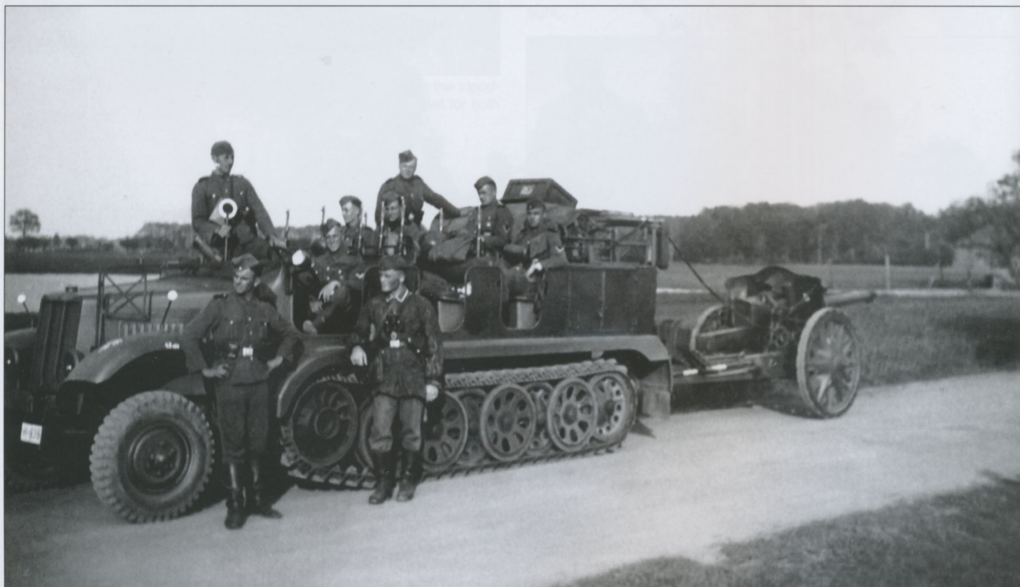
This full nine-man 10.5cm IFH18 light field howitzer crew poses aboard its 5-ton SdKfz 6 medium halftrack. The crew consists of a gun leader (Geschützführer), seven canoniers (Kanoniere), and a motor vehicle driver for tractor vehicle (Kraftwagenbegleiter für Zugkraftwagen). The 3-ton SdKfz 11 was also used to tow the 10.5cm howitzer.
