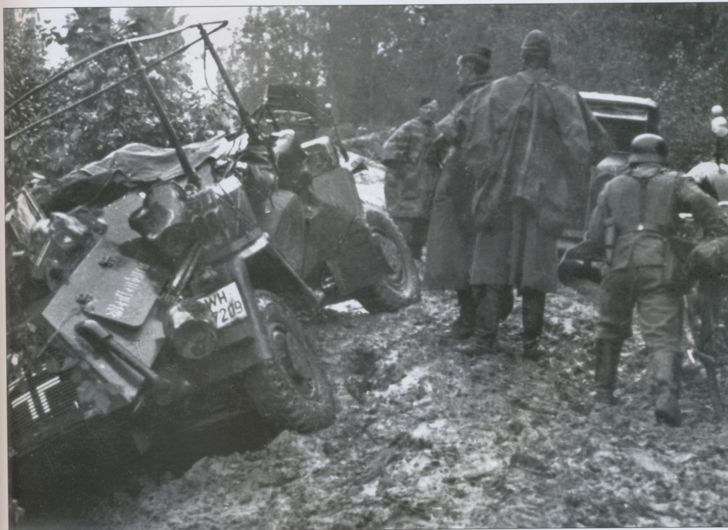
The third armored car of a reconnaissance battalion was an SdKfz 223 Funkwagen (radio vehicle) or leichter Panzerspähwagen (Funk) (light armored reconnaissance car [radio]). It had a folding "bed frame" antenna, which could be lowered to reduce its profile, when traversing through areas with low tree limbs, and during rail transport. It was armed with a 7.9mm MG34 machine gun. The Funkwagen accompanied the other two scout cars to report intelligence information back to the battalion. It had a crew of four.
