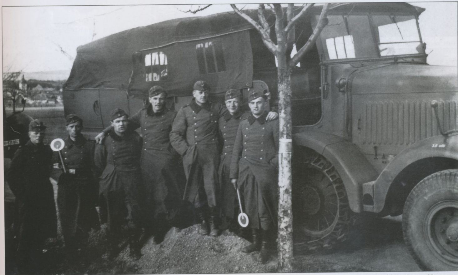
Artillerymen pose beside their 12-ton SdKfz 8 heavy halftrack. This vehicle was used as a prime mover for 10cm guns, 15cm field howitzers, 15cm guns, 21cm mortars, and 8.8cm and 10.5cm Flak guns as well as for pioneer bridging equipment trailers. The red and white signal paddles were carried to send commands and directions between vehicles.
