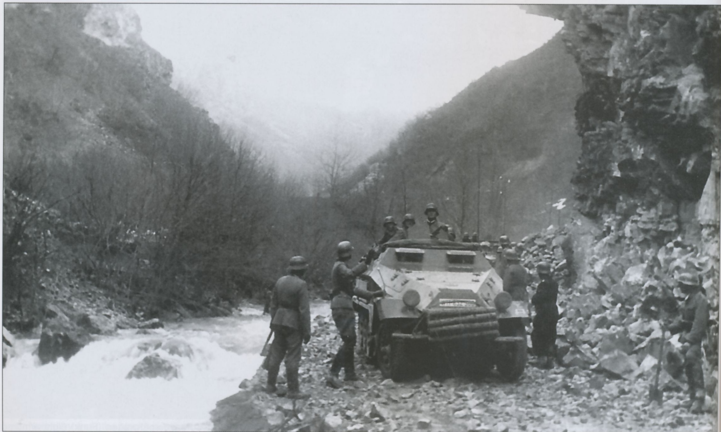
An SdKfz 251/1 armored personnel carrier test drives a streamside road widened and improved by pioneer troops in the Stara Mountains. The half-tracked Schützenpanzerwagen (rifleman's armored vehicle or SPW) was not widely available at this time. The short logs lashed to the front are aid when crossing small ditches and holes plus provide a limited degree of protection from small arms fire.
