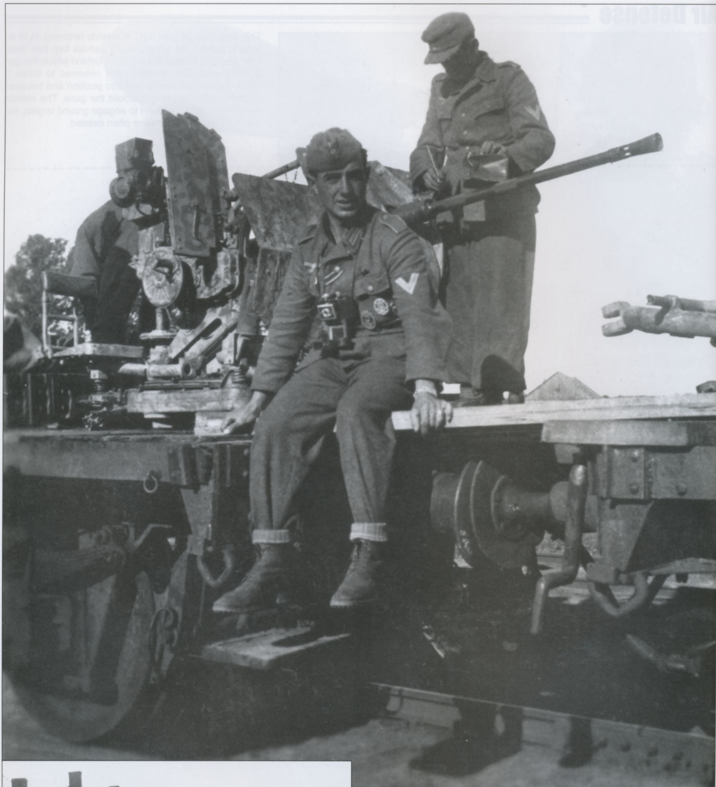
A 2cm Flak 38 has been mounted on a flatcar for air defense complete with its shields. The small camouflage pattern is essentially worthless as from and even short distance it will appear as a single color.
