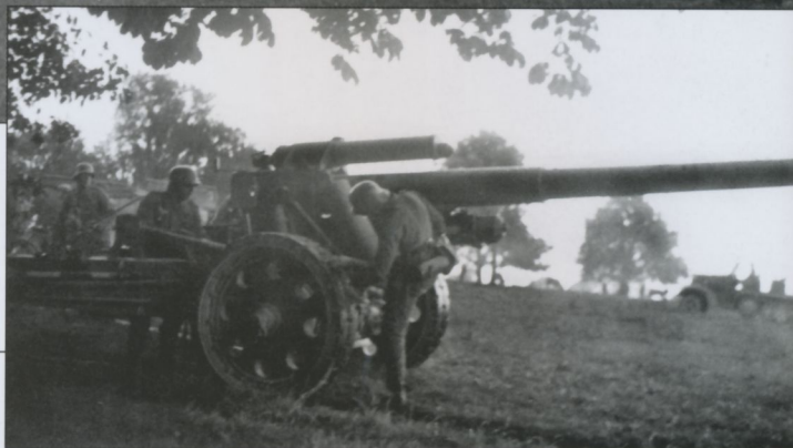
A 15cm sFH18 howitzer is unlimbered and prepared for firing. In the background can faintly be seen a 12-ton SdKfz 8 heavy halftrack prime mover for one of the battery's other howitzers.
