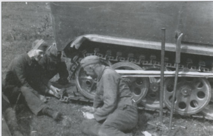
Crewmen of a halftrack replace a broken track link, a labor intensive task. A pry bar and adjusting tools are to their side.
