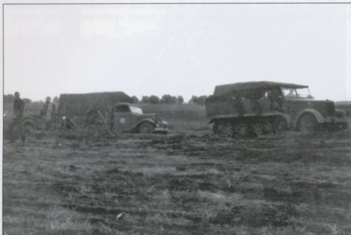
A 12-ton SdKfz 8 heavy halftrack tows a cargo truck out of a mud-saturated stretch of road beside a plowed field. The truck bears a medical red cross on a white disc, but appears not to be an ambulance. It is probably a medical unit's supply truck, especially since it's towing an Sh Ah 401 field kitchen, what the troops called a Gulaschkanone (goulash cannon) or Futterkanone (fodder cannon).
