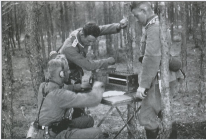
Two NCOs wait to be connected to a subunit by field telephone. A switchboard operator, called a Strippenzieher (line-plugger), makes the connection. The kleiner Verteilerschrank für 10 Leitungen (small switchboard for 10 lines) required a separate field telephone for the operator rather than an integral telephone. The telephone is the Feldernsprecher 33.
