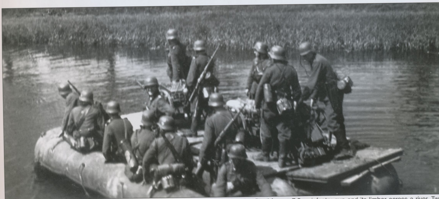
Using two medium pneumatic boats secured side-by-side with a bridge decking section fitted ferry a 7.5cm infantry gun and its limber across a river. Two 7.5cm leIG 18 light infantry guns were usually attached to each battalion from the regimental infantry gun company. Many newly raised divisions lacked these support weapons though.
